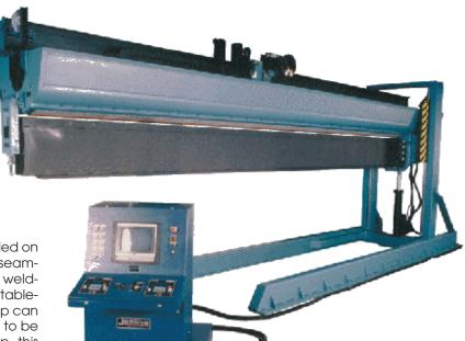
The model illustrated is shown complete with Dual-Arc $^{\text{TM}}$  Plasma/TIG welding capability. It has a weld length of 312" (8 m) and can be elevated to accept cylinders up to 8 ft (2.4 m) diameter.
