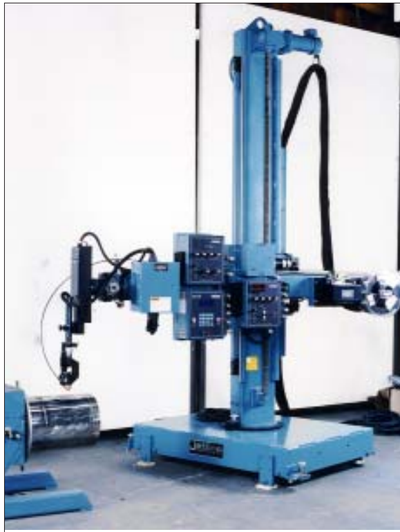
WHL-4C6X6KC with kingpin car Equipped with 9500 microprocessor-controlled plasma welding system
